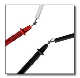
Wrap black and white lead wires from 120V mats, or black and red lead wires from 240V mats around the multimeter probes (color of probe does not matter). Avoid touching the probes during measurement as it could affect the accuracy of the resistance value.
