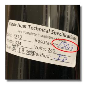
Compare the resistance with the value on the factory label. If the difference is within a range -10%/+5% the mat is okay to use. You can consult chart for lower & upper limits.
