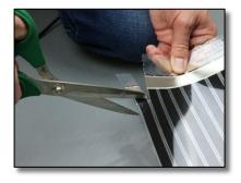
Cut through the last black heating element bar to remove the end of the silver bus bar, creating a notch. Do not over-cut into the next black bar. Repeat on both sides.
