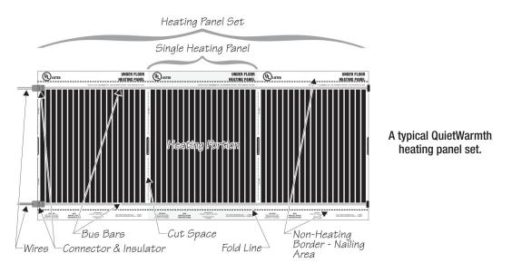
The QuietWarmth System is available in three standard lengths (5', 10', and 15'), and 120V standard voltage. The following table shows the maximum number of single panels that a thermostat can control. If your project requires more single panels than indicated in the table below, additional thermostats or power modules will be required:
