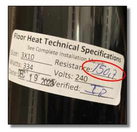
Compare the resistance with the value on the factory label. If the difference is within a range -10%/+5% the mat is okay to use. You can consult chart for lower & upper limits.
