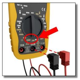
Wrap black and white lead wires from 120V mats, or black and red lead wires from 240V mats around the multimeter probes (color of probe does not matter). Avoid touching the probes during measurement as it could affect the accuracy of the resistance value.
