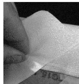
End tape showing Glass cloth electrical insulator
